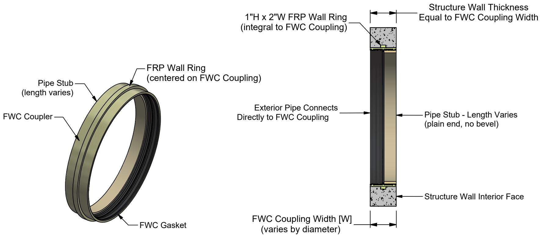
Installed Section View
